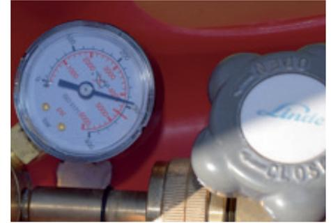
Turn pressure adjust knob on regulator until output gauge shows 4 barg (minimum for BOC's HYMERA® fuel cell).
