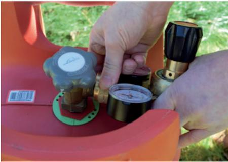
To connect the GENIE® hydrogen cylinder to your fuel cell application you will need a gas regulator to take the high pressure gas from the cylinder down to a low pressure (typically 5 barg) for your fuel cell. BOC supplies a range of GENIE® hydrogen regulators for most applications and no specialist tools are required to make the connections. Note: hydrogen threaded connections tighten anti-clockwise (the opposite to 'normal' threads) as they are left-handed threads
