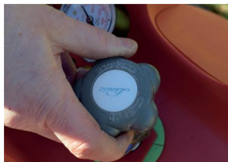
Slowly open the valve on the top of the GENIE® hydrogen cylinder until it is fully open and then turn back half a turn. Check that the contents gauge on regulator shows approximately 300 bar (for a full cylinder).
