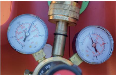
**IMPORTANT** – both gauges should now indicate zero. If there is any pressure left in the system it will be impossible to undo the regulator.
